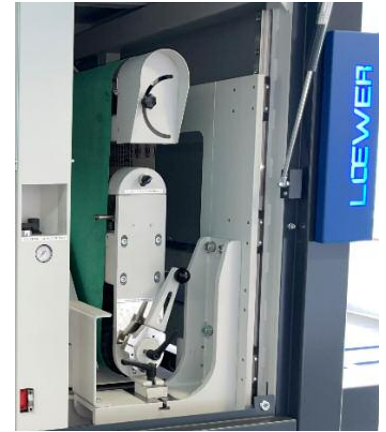
Abrasive belt unit with floating head system
